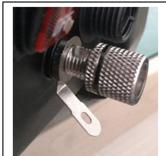
Step 1: unscrew the knob on the rear of the drive; do not unscrew the part fixed on the housing, as shown in above picture.
