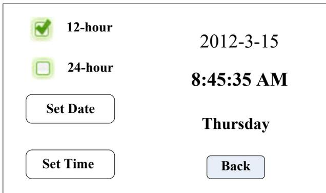
In this interface, you can set the current date and time, and it will display at the top right of corner. Click the **Set Date** button, and out comes the **Set year** numeric keypad, the range of the year is **1970-2099**. After setting up the year, then set the month and date.
